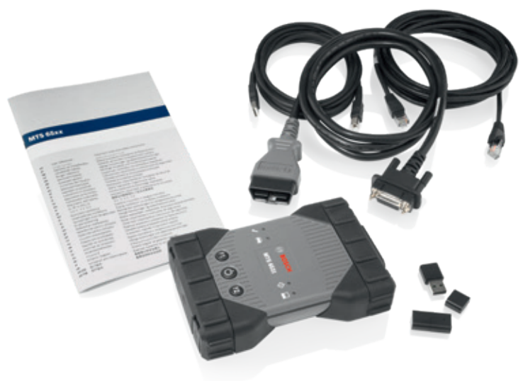
MTS 6531 with P2P Wi-Fi: kit contents
